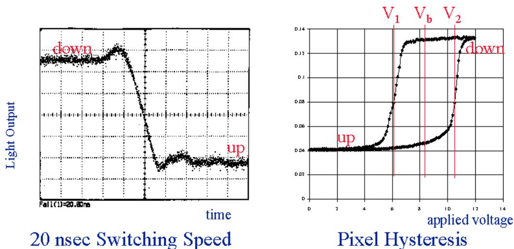
Figure 5: To switch a ribbon down requires a voltage differential of  $V_2$  volts or more between the ribbon and a bottom electrode. The ribbon will remain down until the voltage differential falls below  $V_1$  volts. This ribbon hysteresis offers mechanical memory and zero-power pixel-state retention. Switching time is approximately 20 nanoseconds.
